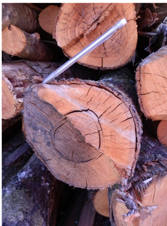
Figure 2. Reject chestnut logs in the open-air storage. One can clearly see the central log as being affected by ring shake, which rules out its conversion into a high-value fencing product.
