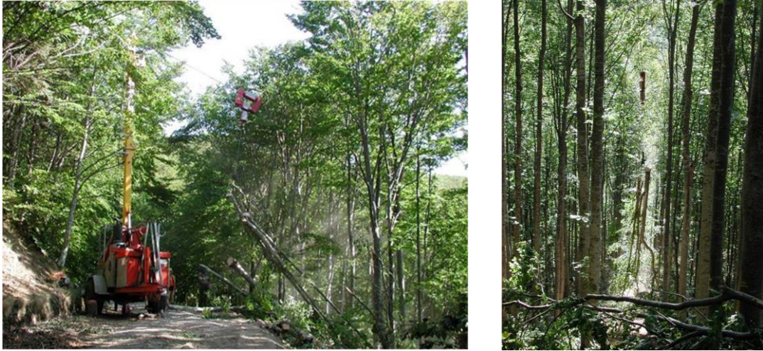
Figure 3. One of the cable yarding operations common on the Pistoia mountains. A light tower yarder is used to bring whole trees to the roadside, where they are processed and loaded on trucks for subsequent transportation to the end user or to a centralized sort yard.
