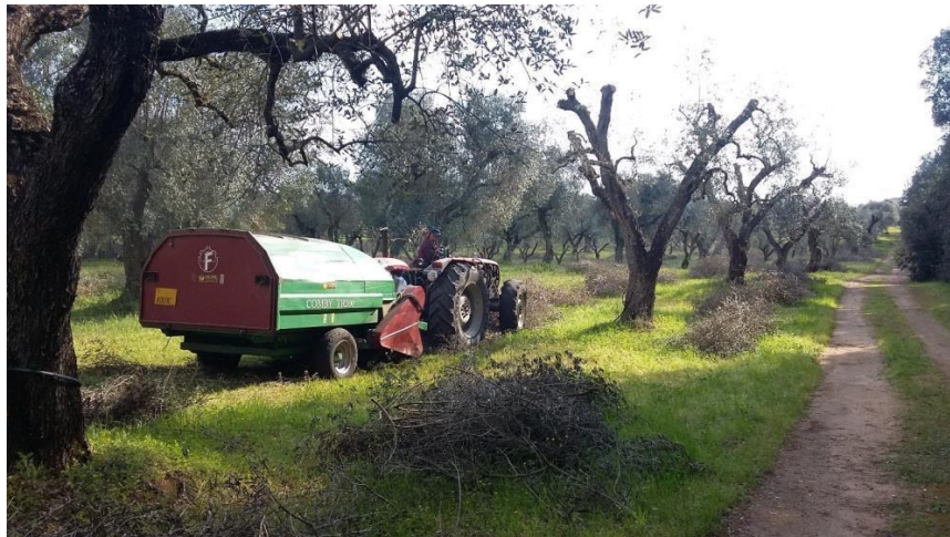
Figure 2 - Harvesting of pruning residues with a four towed shredder (Facma mod. Comby TR200) for olive groves with less than 400 trees
