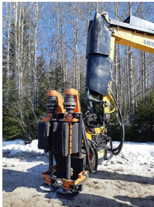
Figure 1. RISUPETO harvesting device suitable for mobilizing forest biomass from young or unmanaged thinning stands.
