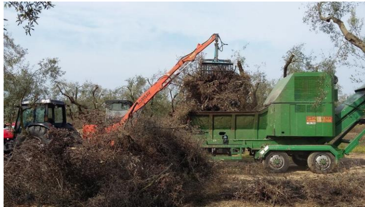
Figure 3 - Comminution of pruning residues with a mobile shredder (Caravaggi mod. BIO900) for bigger olive groves
