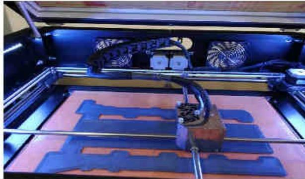
The printer uses the Cartesian movement for the X, Y axes with a static support mechanism composed of 12 mm INA cemented linear bars and for the dynamic support of self-lubricated linear bars 10x2 mm each.
