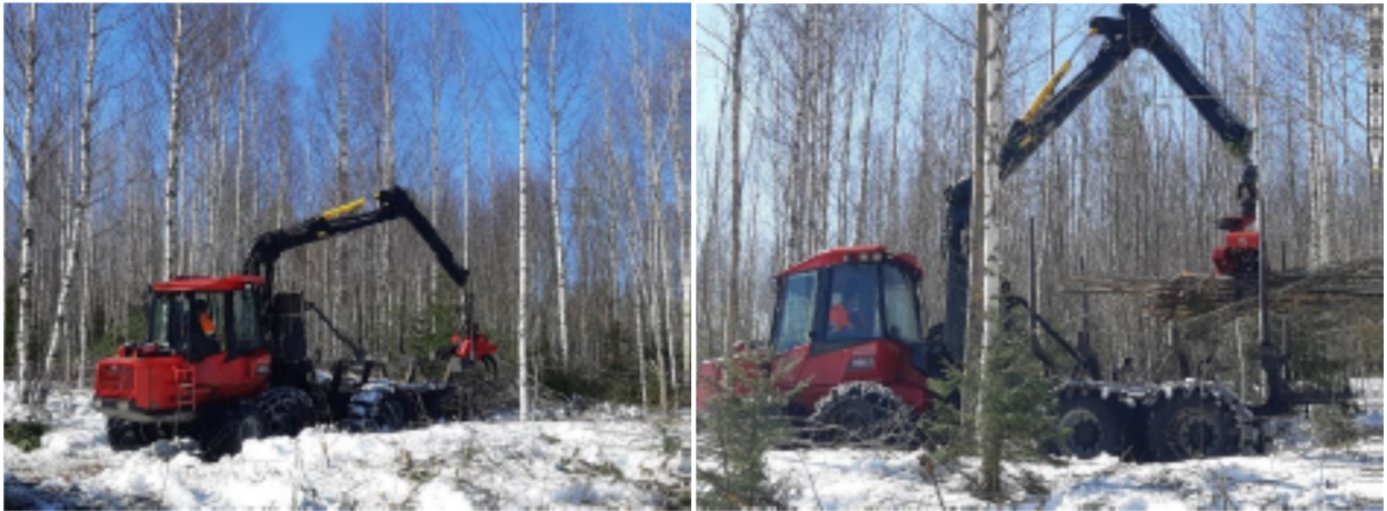
Figure 3. Collection of forest biomass from thinning using a forwarder..
