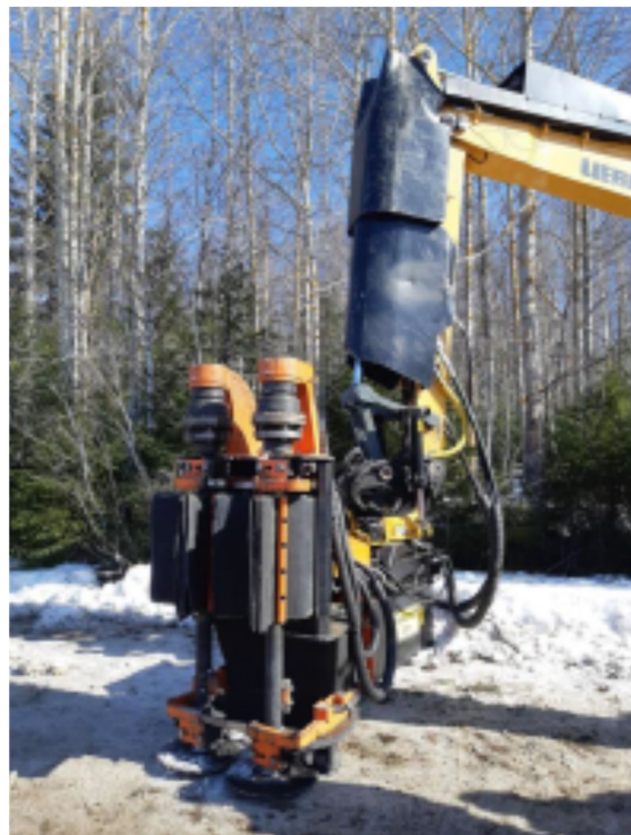
Figure 2. RISUPETO harvesting device suitable for mobilizing forest biomass from young or unmanaged thinning stands.
