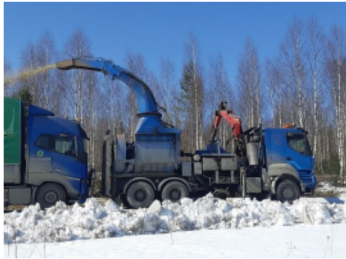
Figure 5. Chipping of biomass using a truck-mounted drum chipper.
