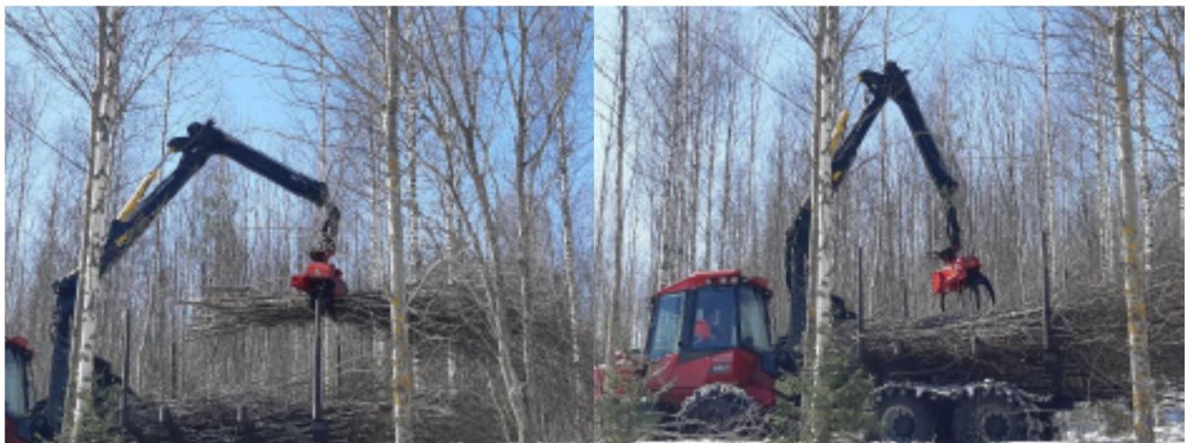
Figure 4. The forwarder is equipped with a Mecanil grapple saw.
