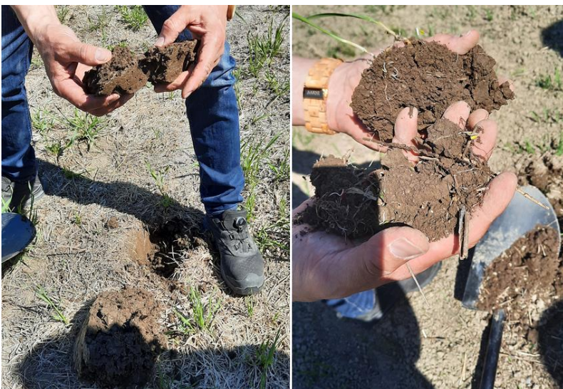
Figure 1. The soil before (left) and after (right) experiments where different organic soil amendments were added to soil to improve the structure of clay soil. Photos: Saija Rasi.
