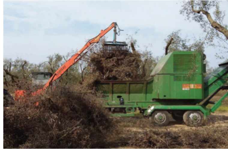
FIGURE 3. Comminution of pruning residues with a mobile shredder (Caravaggi mod. BIO900) for bigger olive groves
