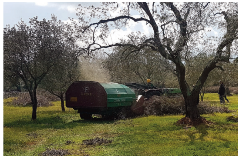
FIGURE 2. Harvesting of pruning residues with a four towed shredder (Facma mod. Comby TR200) for olive groves with less than 400 trees
