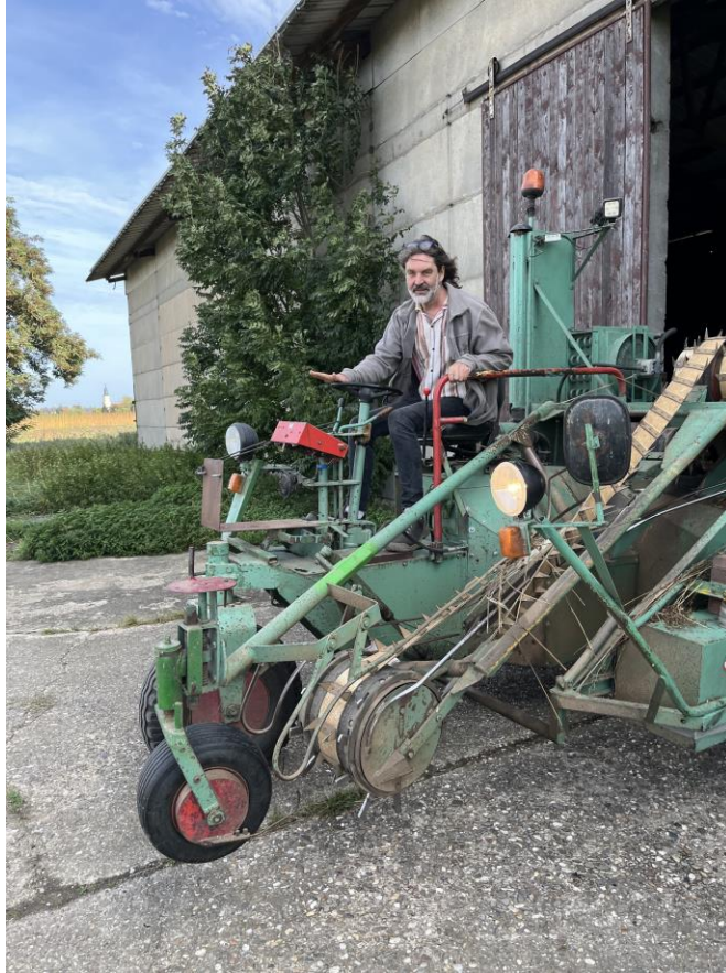
Picture: Machinery to turn the hemp stems on the field.
