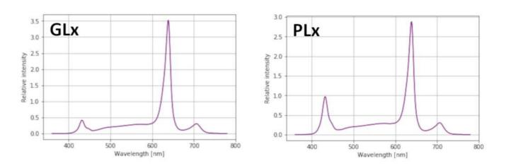
SCORPIO SCR-2CH and 4CH are LED fixtures with adjustable spectrum with 2 and 4 indipendent dimmable channels. See the chart below for channels definition.
