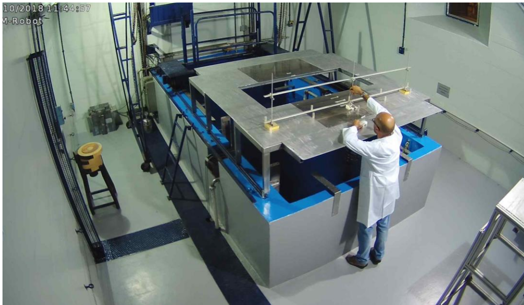
Figure 5 - Irradiation cell view and movable supports for dosimetric measurements.
