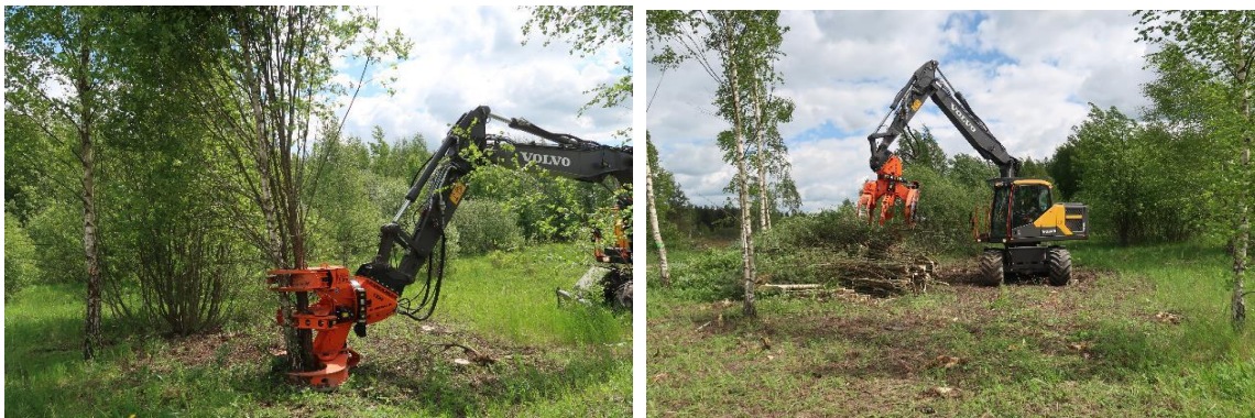
Felling trees, bushes using a Westtech Woodcracker hydraulic shear head
