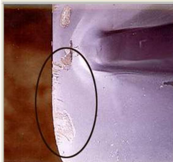
This stern drive cavitation plate was lightly scraped by a fork lift truck. With the aluminium exposed, the metal now begins to erode strictly as a result of stray current which has left the metal bright.
