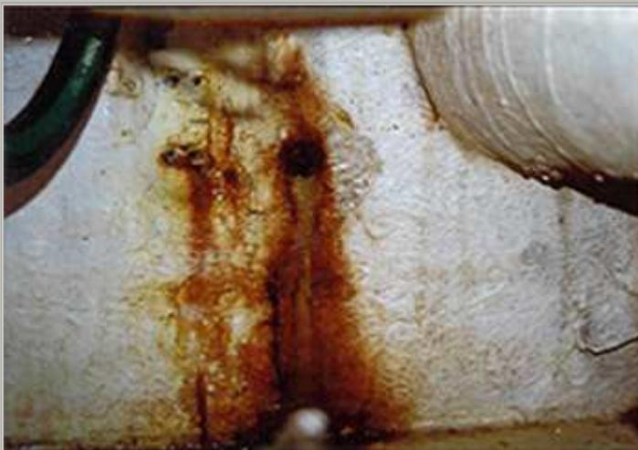
**This is one of the telltales of crevice corrosion in through hull bolts. The fact that this is Taiwan stainless only makes the problem worse.**
