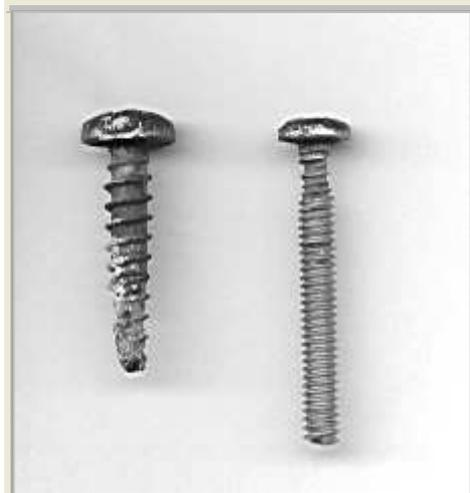
**Crevice corrosion on screws. The one on the right shows the typical wasting of the shank right under the screw head. The one on left was exposed to water both under the head, and on the inside of the hull where it has thinned at both locations. This is probably what the bolt in the photo below (top) would look like when removed.**
