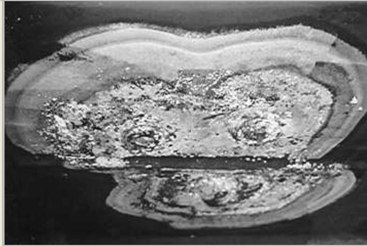
This is what copper-based paint looks like when stray current is involved with these through hull bolts. The copper-based paint has reacted. You can't get a better indicator of a problem than this.
