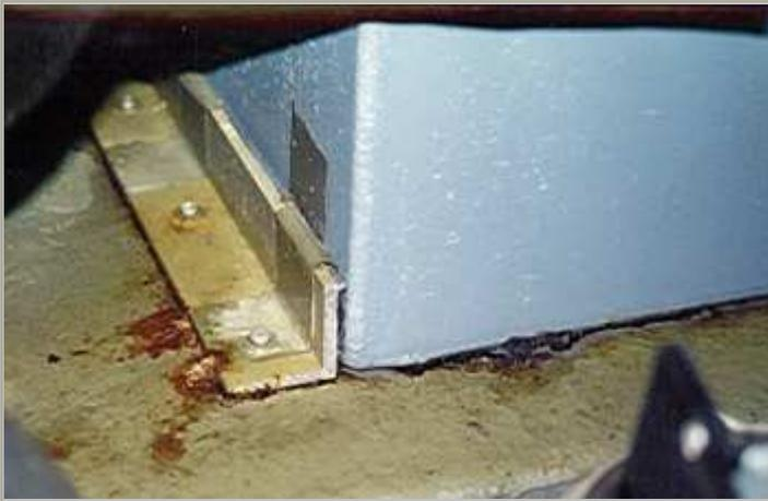
This is how you can tell if your going to have an aluminium fuel tank problem. Sitting on a flat deck that gets wet, here you can see the corrosion stains coming out from under the tank. This one's days are numbered.
