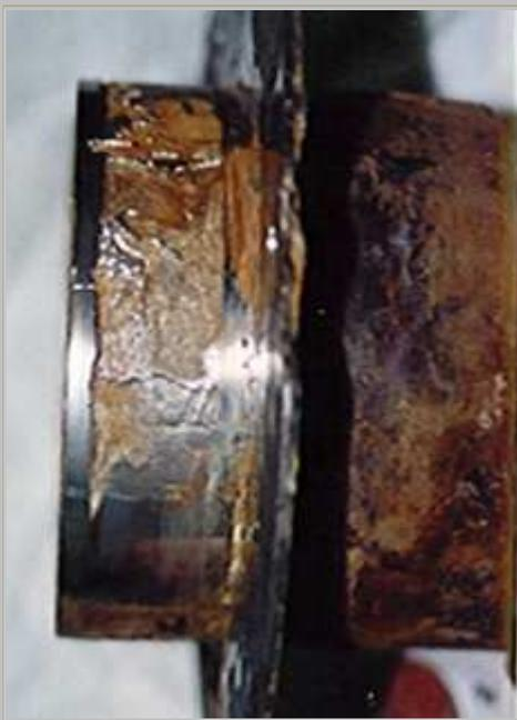
**Classic crevice corrosion. In this case caused by a carbon rubber exhaust flapper clamped onto a stainless exhaust flange plate. Notice that the worst corrosion is where the clamp pressed the rubber the tightest.**
