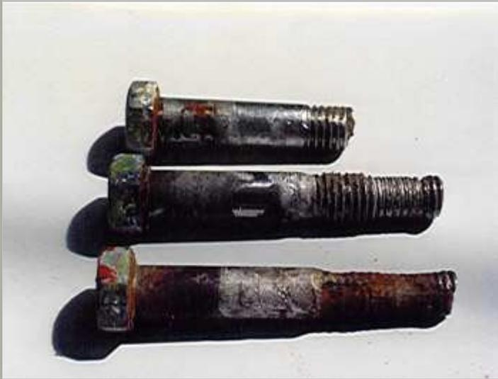
Crevice corrosion of through hull bolts. In this case, the water got at the bolts from the inside. The use of nuts with nylon inserts (shake proof type) accelerated the process. Notice that the acid etching leaves the metal very bright. This is a total lack of oxygen to the cavity, whereas the exposed threads look rusty and had more oxygen available. That's because the nut completely wasted away.
