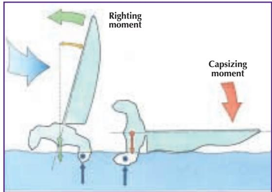
**It is therefore vital that the amount of sail carried is not sufficient to cause capsize, even in a gust,** which may cause a doubling of wind heeling moment.
