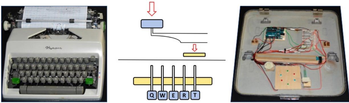
**Figure 2:** From left to right: the Olympia SM9 typewriter used in the CS1; the sensing mechanism - by pressing a key (blue) the metal bars touch the potentiometer (yellow) in a specific point; the Olympia SM9 suitcase base equipped with Arduino, sensors and LEDs
