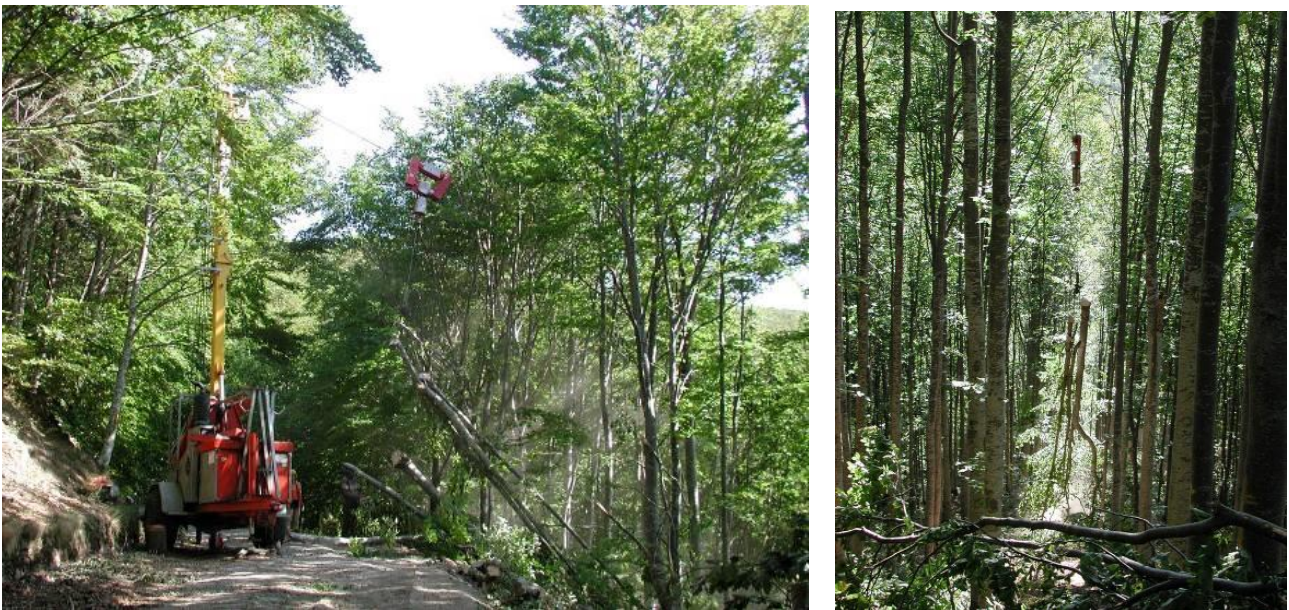
Figure 3 – One of the cable yarding operations common on the Pistoia mountains. A light tower yarder is used to bring whole trees to the roadside, where they are processed and loaded on trucks for subsequent transportation to the end user or to a centralized sort yard.
