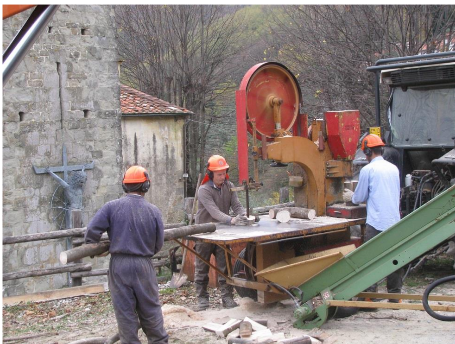
Figure 8 – Traditional semi-mechanized firewood processing is labour-intensive, costly and hazardous
