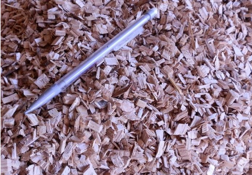
Figure 1 – A classic example of microchips, produced here as a pellet surrogate to feed small-scale pellet stoves for residential use. This product must be very small ( \leq 7 mm), very even and very dry ( \leq 13\% on a wet weight basis). Otherwise, the stove may malfunction...
