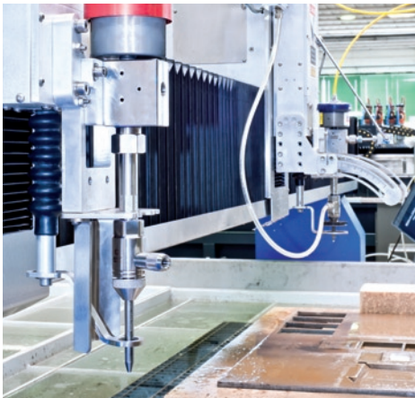
MMC - Multiple Master Carriage Carrelli master multipli controllati da CNC. Multiple Master transverse motorized carriages.
