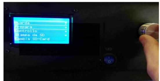
The printer can be used via USB connectivity with computer or via SD card to print independently. There is the possibility to control with the supplied tablet, remotely the printer using the webcam with dedicated IP address. An application for controlling and managing print parameters is installed inside.
