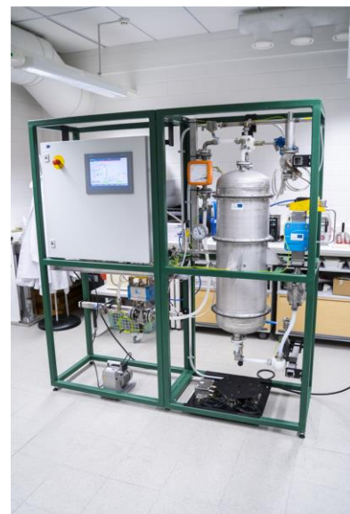
Biomethane liquefaction unit. Source: Centria UAS
