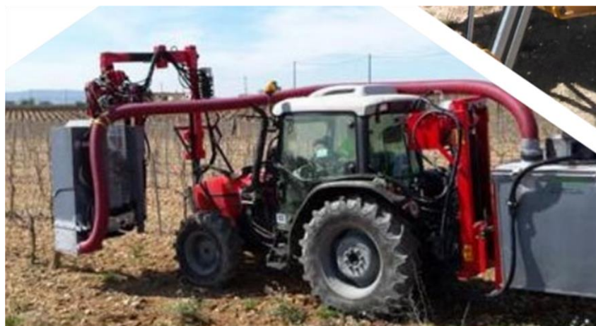
Figure 1. Prototype developed to collect vineyard pruning.
